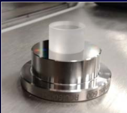
Fig. 1: molding form made of Inconel 600, right
