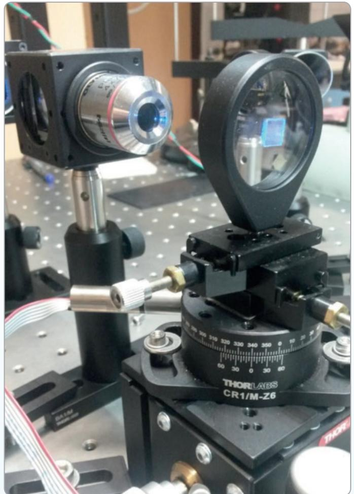
*Figure 1: Barium titanate single crystal in the sample holder with transparent electrodes fixed in the rotating stage of the digital holographic tomograph.*
