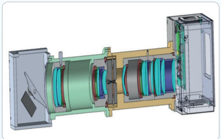
complexity of the optical system increased requirements on production and accuracy of assembly. Special care was taken to optimize the shape of the optical elements with respect to available production technology (in this case, the SPDT – Single Point Diamond Turning – method).
